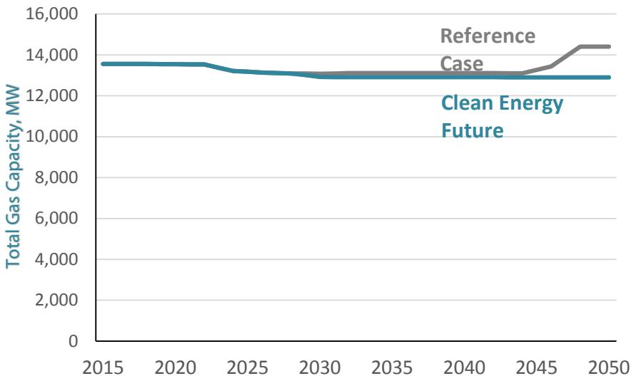
Figure 2-4. Natural gas power plant capacity in Illinois, 2015-2050
